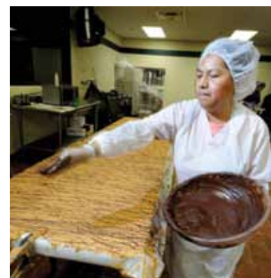
Pumpkin bark production involves adding ingredients such as graham cracker crumbs, dried pumpkin, ginger, allspice and nutmeg, into a mixer. After mixing, pouring onto a table, leveling and then drizzling of chocolate, the pumpkin bark is placed into a cooler.
