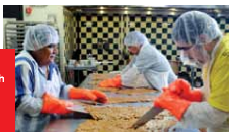
Peanut brittle production at Long Grove Confectionery begins in the kitchen area with cooking, followed by pouring out the candy mass onto a cooling table. Hand forming and scoring completes the first stage.
